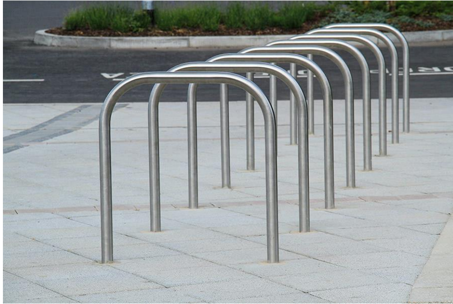
Figure 17 – Photo of sheffield stands 23
